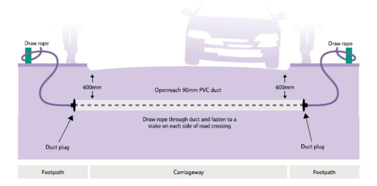
Duct laid beneath a carriageway crossing must be 600mm depth from the cover of the final surface levels and, for engineering reasons (National Joint Utilities Group NJUG), separated from other services laid in parallel by 600mm (to permit us to install underground joint boxes without the need for bends). Cable marker no.2 is needed at the site entrance/boundary, to ensure link up identification for our contractors.
